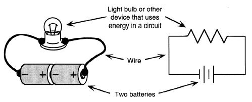
Using a bare bulb (out of its socket), one battery, and **two** wires, try lighting the bulb in as many ways as you can. On a separate sheet, sketch at least two *different* arrangements that work. Also sketch at least two arrangements that don't work. Be sure to label them as "works" or "doesn't work."
