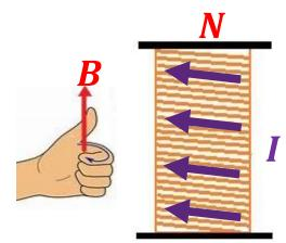
South pole of the magnet faces downward, then the top end of the coil will act like a S pole requiring that the thumb of the left-hand points downward and the electron flow is reversed.
