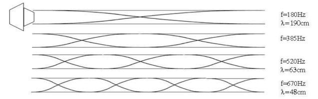
The fundamental mode (top diagram) is difficult to detect well. The higher harmonics give more distinct amplitude changes at resonance. The theoretical wavelength for each frequency can be calculated from v=fl using a value of 330 ms<sup>-1</sup> for the velocity of sound in air, v.
