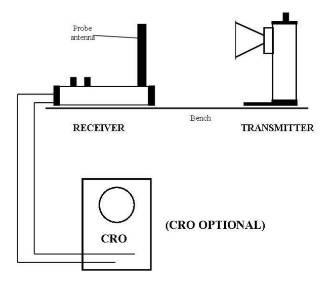
The output from the detector can be taken to an oscilloscope if quantitative measurements are required. Connect the black output socket on the receiver to the negative input on the CRO and the red output socket to the signal input, usually red, on the CRO.
