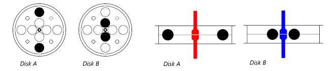
Place 2 steel balls into each disk as shown here. Insert a red axle into Disk A and a blue Axle into Disk B to help reference the different patterns.
