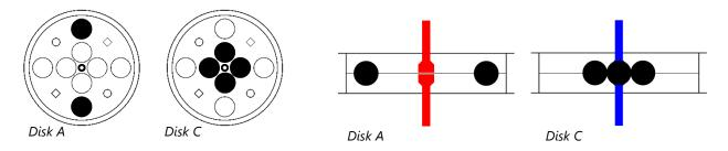
Logically, it seems like the rotational inertia depends on both the amount of mass AND the distance of the mass from the pivot (center).
