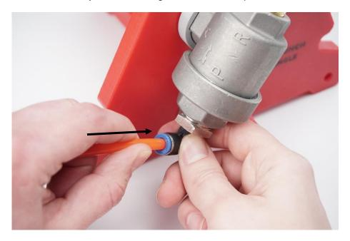
Push the other end of the tube into the slide valve. This connection should also click into place.
