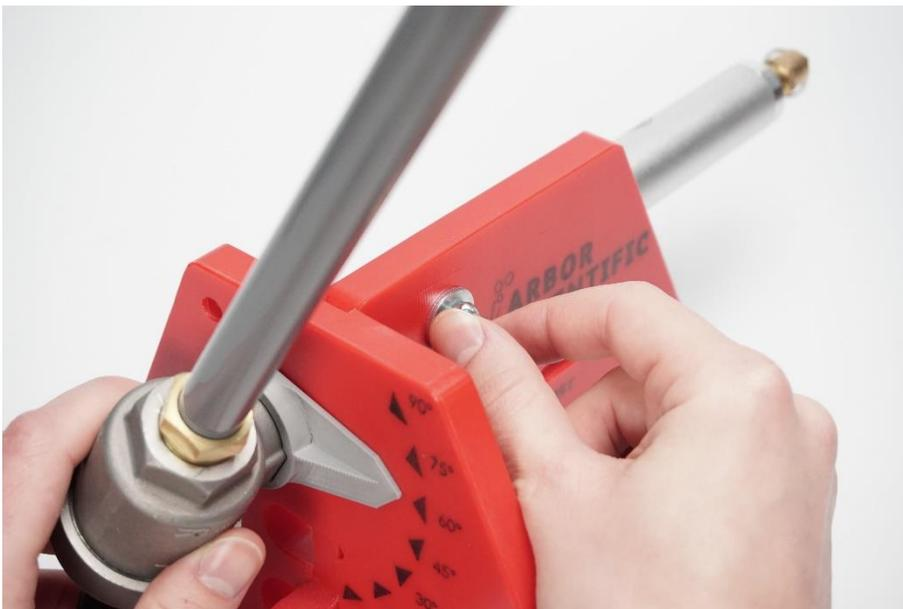
Now simply connect any bicycle pump to the valve on the regulator, pressurize, and launch! Follow instructions in the Teacher Guide for the launching procedure.
