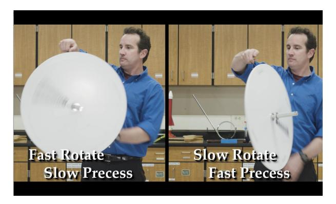
Next, we also note that the location of where the string attaches can affect the rate of precession. This is because the torque from the weight acting on the handle is dependent on the distance. Demonstrate this by moving the hook nearer to the axis. Now the wheel will almost not precess at all. This teaches us that it really is torque that causes the precession.
