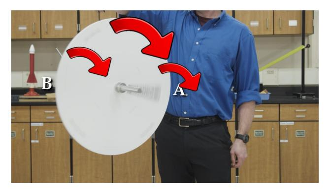
We imagine a point of the wheel that moves from A to B in the figure above. As it moves it is subject to the tipping torque from the wheel itself which wants to flop forward under its own weight. This torque accelerates the point to the right. But it takes time to get faster. Thus, when we finally get from A all the way to B we are now ready to move to the right, which is exactly what happens. Point B moves to the right and point A moves to the left. Try it for yourself!
