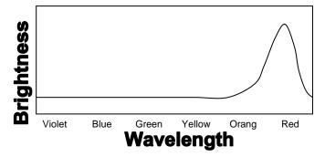
Notice that the transmitted light is brightest near the red part of the spectrum. The rest of the wavelengths have low brightness. Here are the transmittance spectrums of the 6 color filters included in the kit. They refer to wavelength in nanometers along the x-axis. Rather than using brightness or amplitude, the graphs refer to the transmission, or the percentage of the original brightness that was allowed to pass through, along the y-axis.
