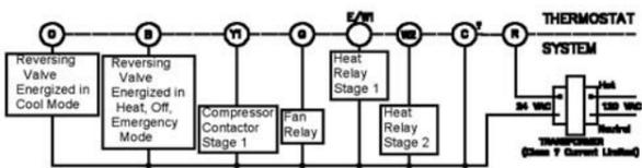
Figure 6. Typical wiring diagram for single transformer multi-stage systems
