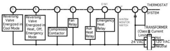
Figure 3. Typical wiring diagram for single transformer heat pump systems
