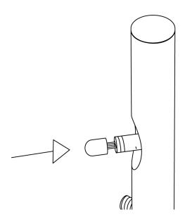
2. Twist glass orbs onto threaded rods
