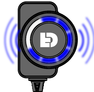
Flashing Blue LEDs Light Circuit One fuse setting mode
