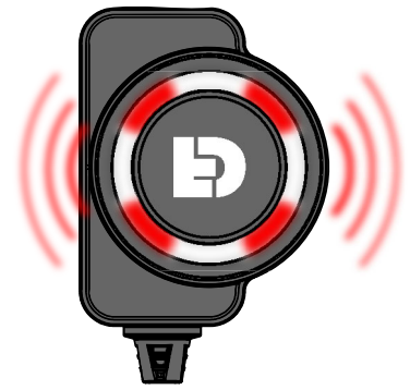
4 Flashing Red LEDs Vehicle battery voltage below 10.8v
