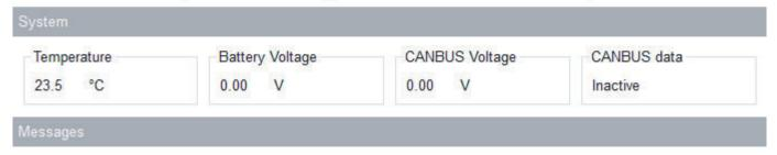
No CANBUS voltage detected. This could be due to a faulty connection or ignition is off.
