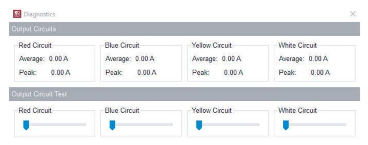
Use the sliders to test circuits. Closing the diagnostics window will revert back to normal operation.
