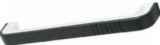
45 749 1508 Decorator handle, 305mm (12") K Line, heat resistant, aluminium, nylon bases, hole centres 270mm (10 5/8")
