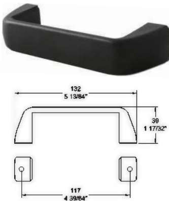
46 2248 Black thermoplastic (-40°C to +130°C), 117mm (4 39/64") hole centres M8 Thread
