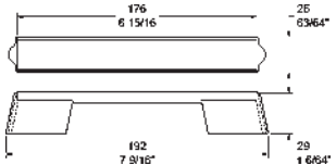
45 749 1506 Decorator handle, 176mm (7") K Line, heat resistant, aluminium, nylon bases, hole centres 153mm (6 1/32")
