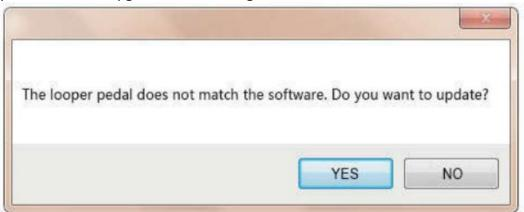
c) After the upgrade is complete, you will enter the normal user interface. Use the IMPORT button to download files from the computer to the pedal. Use the EXPORT button to upload recorded data from the pedal to the computer. (Currently,
