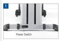
STEP 1. Turn the power switch to the "Off" position on the back base of the PowerTower unit.
