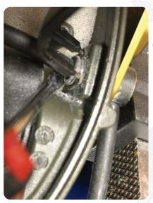
4 It is recommended to use a small punch or screwdriver to help hold the snap ring in place during install. This is the probably the most frustrating part of the SARA<sup>TM</sup> install process because of the tight work space. Take your time and ensure the snap ring is fully seated in the groove around the stud. Once satisfied that it is properly seated, use the snap ring pliers to close up the ring as much as possible.
