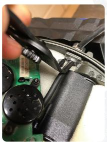
The vise helps relieve pressure on the studs, freeing up the snap rings for easier removal with snap ring pliers.
