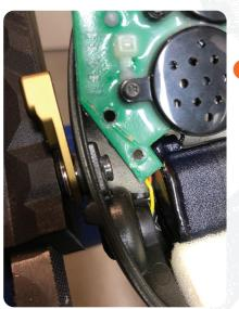
3 Once OEM headband wires have been removed, replace with SARA's™ and reinstall studs in housing. Place the new assembly back in the vise. The pressure will help to expose the recesses in the studs where the snap rings will
