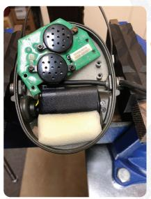
MSA/Sordin<sup>™</sup> headsets were never designed to be disassembled. This process can be a little tricky and frustrating without the right tools. Installers will most likely need both hands. It is recommended that the headset ear cup assembly be gently placed in a padded vice to put slight pressure on the studs. This will make removing and installing the snap rings easier.
