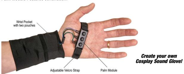
When preparing the sounds you wish to play, please refer to the instructions for the Sound Module. The wires from the Palm Module must be plugged into the sockets marked S1, S2 and S3. The three buttons on the Palm module will activate the sounds stored on the memory inside the sound module. Please note which wires plug into which socket, so you can organise which sounds are played when each button is pressed.
