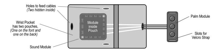
The Wrist Pocket is made from stretch fabric, one size fits all. There are two stretch pouches, one on the front and one on the rear. The Sound Module, Battery Pack and Speaker Module can be stored in either of these pouches. There are holes in the Wrist Pocket that allow you to feed cables through. Please note that there are also two hidden holes inside that allow you to feed wires between the front and rear pouches.
