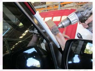
19. Remove the burs from these holes, remove masking tape, paint all bare metal surfaces including the holes drilled in the quarter panel, and remove all metal fillings from the A-Pillar gutter and quarter panel.
