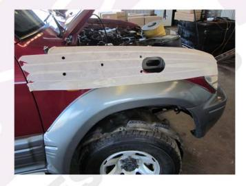
12. Using a hammer and drift, bend the lower section of the inner guard bracing in, this will allow clearance of the snorkel body outlet.
