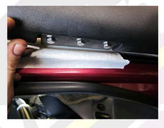
16. Remove the snorkel body, remove the upper bracket and position on the A-pillar in the position marked in step 15, and mark the 4 mounting holes.
