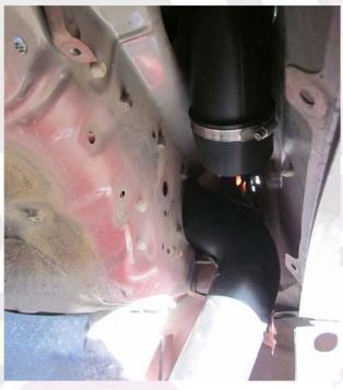
26. Remove the original air box to intake adaptor by drilling out the 2 rivets and remove the metal filings.
