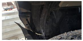
For the LH side cut the guard slightly longer and bolt to the rear of the bash plate on the inner hole, then trim flush with the bottom of the bash plate.
