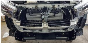
17. Trim the original LH and RH vertical air dams as seen in the photo below to clear the new mounting bracket and bullbar.
