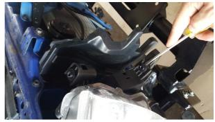
20. Drill a small hole in the air damns just in front of this to attach a cable tie to, and cable tie it to stop movement.
