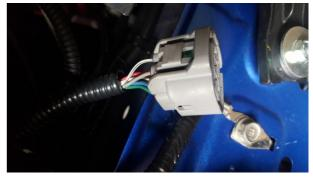
27. For the indicator positive feed, there is a small conduit that goes up into the back of the indicator, this can be pulled down below the headlight and the red wire on the right hand side used, and the yellow on the left hand side (Australian vehicles) NOTE: you must double check this with a multimeter or test light to confirm.
