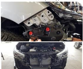
14. Install the inner and outer bullbar bracket supports to each side of the chassis using the M12 fine bolts with washers for the rear 2 outer mounting points. The longer bolts pass through the chassis through both brackets. Use a washer on each side. Leave bolts loose for now.
