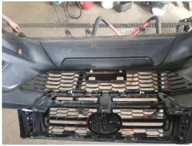
Remove the front horizontal air dam and the LH and RH vertical air dam, keeping aside for re-fitment later.
