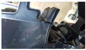
21. Install the new grill support bracket. It is recommended to remove the screw plug and use a nut and bolt to tighten it correctly. The grill bracket will point upwards and screw to the back of the Toyota badge.
