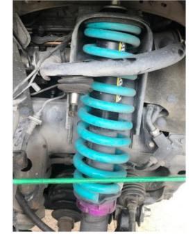
3. Using OE bolts and supplied bush washers (two per UCA) loosely bolt the Dobinsons UCA into the OE chassis mounts, using the Left and Right arms. Fit the supplied washers to the outside of the arms (outsides of either end bushes). This should look like the OE fitment.
