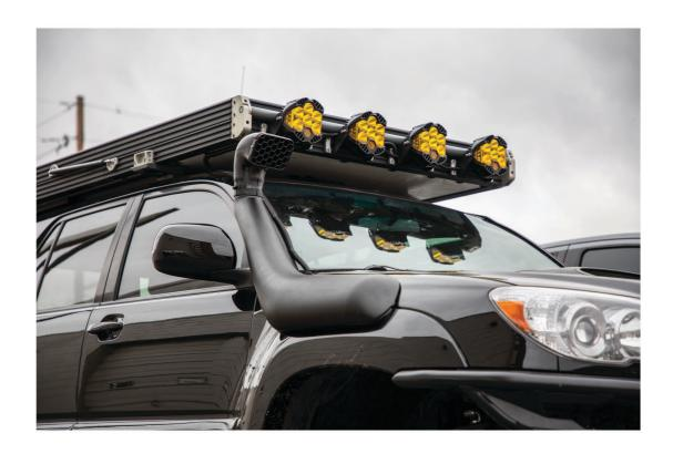
This Snorkel will take approximately 3 hours to install and is installed to the Righjt Hand Side of the vehicle.
