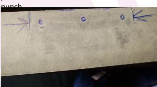
21. Pilot drill the holes, and then drill to suit the rivets supplied. It is a good idea when doing this to drill through a block of wood or equivalent spacer so that only about 5mm of the drill tip sticks out so you do not drill through your interior or air bags.
