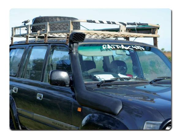
This Snorkel will take approximately 2.5 hours to install and is installed to the Right Hand Side of the vehicle.
