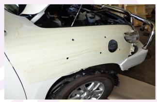
10. Then using the Pneumatic hacksaw or small metal cutting jigsaw cut away the section as seen on page 2.
