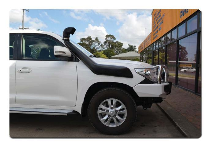
This Snorkel will take approximately 3 hours to install and is installed to the Right Hand Side of the vehicle.
