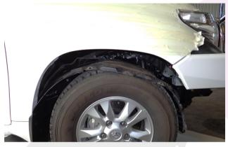
3. Remove the plastic air box joiner located above the inner wheel arch and keep bolts.
