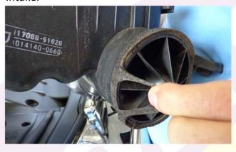
20. Turn the dust valve to closed as seen the in picture above and seal the small hole in the bottom with sealant.
