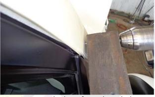
17. Remove the burs from these holes, remove masking tape, paint all bare metal surfaces including the holes drilled in the quarter panel, and remove all metal fillings from the A-Pillar gutter and quarter panel.
