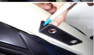
16. Pilot drill the holes, and then drill to 7.5mm. It is a good idea when doing this to drill through a block of wood or equivalent spacer so that only about 5mm of the drill tip sticks out so you do not drill through your interior or air bags.
