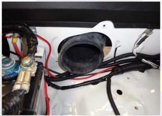
29. Re-install the airbox aligning the air-box intake with the rubber joiner. Tighten both hose clamps.
