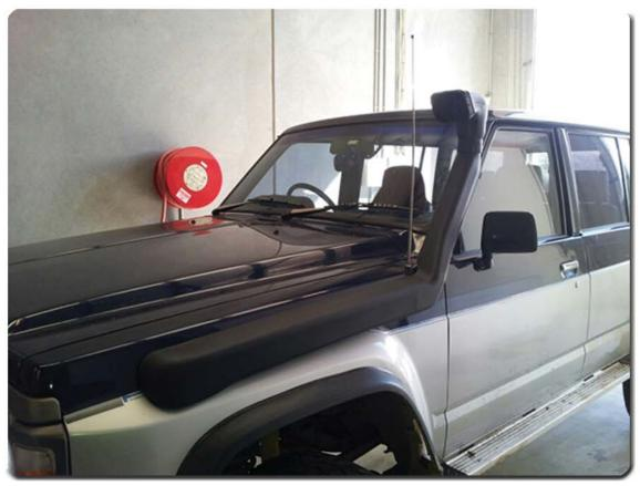
This Snorkel will take approximately 2.5 hours to install and is installed to the Left Hand Side of the vehicle.
