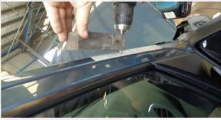
19. Remove the burs from these holes, remove masking tape, paint all bare metal surfaces including the holes drilled in the quarter
