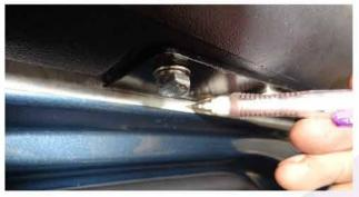
16. Remove the snorkel and remove the top mounting bracket from the snorkel body. Place the bracket back into its marked position and mark the holes.
