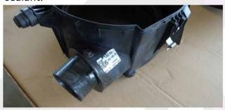
29. There is a small drain valve located under the airbox, Dobinsons also recommend sealing this with sensor safe sealant.
