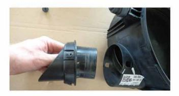
28. Clean the surfaces and apply a thick bead of sealant to the outside of the adaptor, to the screw holes and also to the locking tabs to provide a seal between the airbox inlet adaptor and the airbox.
