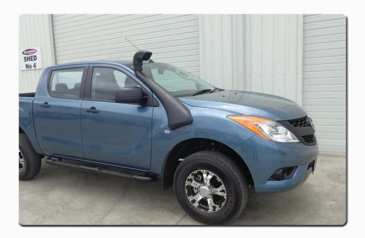
This Snorkel will take approximately 3 hours to install and is installed to the Right Hand Side of the vehicle.
