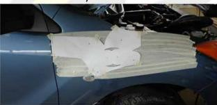
7. Drill the 6 holes with a small pilot drill, then remove template.
