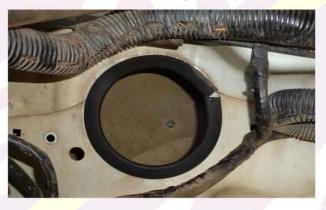
20. Check the inner guard duct large end fits over the snorkel body outlet, you may have to put a small bevel on both pieces to get them to join properly.
