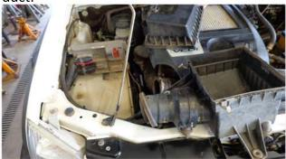
3. Apply masking tape to the RH quarter panel, it is a good idea to cover the whole panel so you do not scratch it when working around it. Carefully unclip the side indicator.
