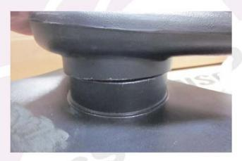
21. Install the inner guard duct supplied into position inside the guard. This can be quite a tight fit. Install the engine bay end first, this is easiest done by having the other end of the duct towards the ground and slightly towards the centre of the vehicle, it can then be rotated until the end of the duct goes through the hole into the engine bay. The other end can then be rotated up into position, aligning it with the guard hole.
