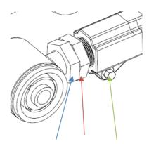
Tighten this nut (blue arrow) against other adjuster (red arrow). Tighten Locking bolt (green arrow)
