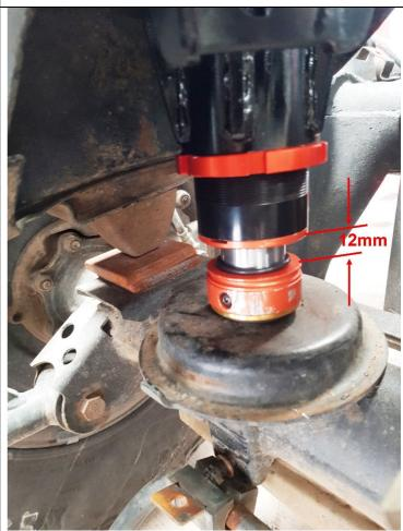
12. Tighten all nuts on bolts aside from the 14mm trailing arm bolts - keep these finger tight for now/
