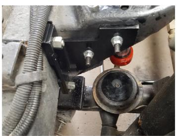
9. On one side at a time, remove the front bolt of the upper trailing arm. Install the longer 14mm bolt supplied with the bolt head on the inside through the arm mount. Then on the outside of the arm mount add the 14mm thick spacer supplied, then the correct side forward running brace then the washer and nyloc nut. Loosely. Install the M8 x 55mm bolt through the angled brace at the front of the arm with the locking nut supplied.
