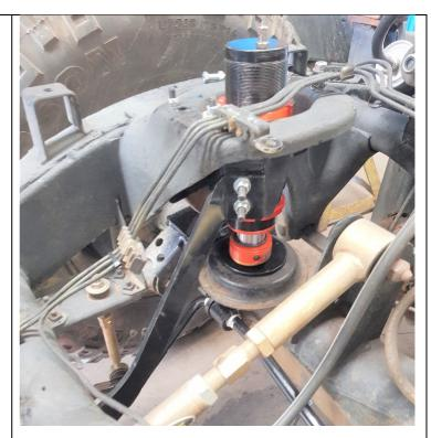
11. Set the bump stop height and lock off the lower locking ring. With the vehicles full weight on the bump stops, the hydraulic bump stop must still have 12mm of exposed shaft. This will close up a little more during large impacts but will not fully bottom the hydraulic bump stop and ensure all remaining force is transferred through the factory rubber bumpstop.
