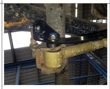
Loosely bolt the front mount to the main bump stop mount using the countersunk bolts, washers and nyloc nuts supplied.
