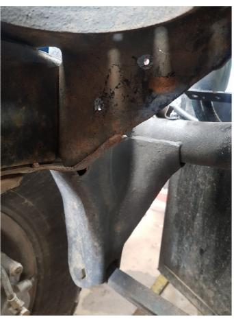
6. Remove the mount and Pilot drill the holes and drill to suit the M10 bolts supplied. A right angle drill attachment may be required. Clean away the drill shavings and paint bare metal surfaces to prevent rust. Repeat on both sides
