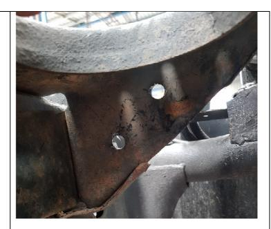
7. Install the lower strike plate to the lower coil seat with the countersunk M10 bolt, sliding up the washer and nyloc nut from underneath and tighten.
