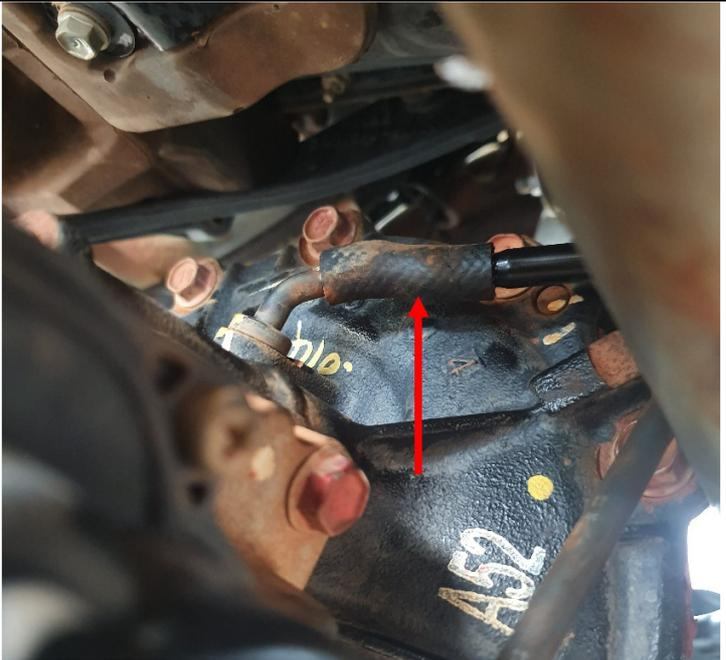
18. Replace the front 4mm i.d. vacuum hose at the front 4wd locking solenoid (for models equipped with this) with the longer hose ensuring it is connected properly at both ends, cable tie both ends with a small zip tie to keep it firm.
