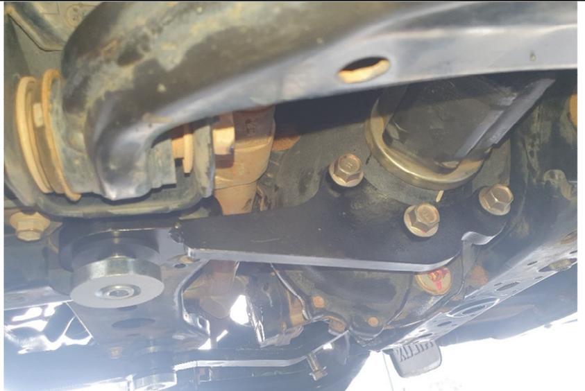
15. Remove the jack and tighten all bolts. The large and small slotted washers supplied are generally not used and provided for customers who wish to raise the rear of the diff slightly to prevent cross member contact.
