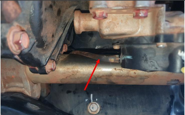
19. If required unclip the wiring retainer from the front left side of the diff if it is over stretched – this is recommended.
