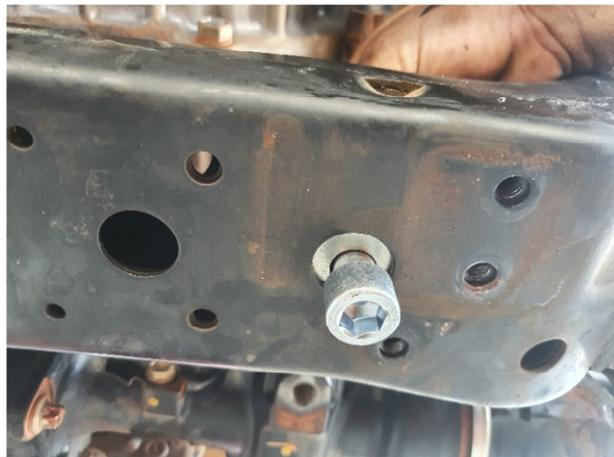
12. Install the new right side cradle to the diff to the bolt installed in the step above. The cradle will only go 1 way with the 2 holes for the diff towards the rear. install in the order as shown ensure that the sleeve goes inside the 60 x 8mm thick washer. Leave loose for now.
