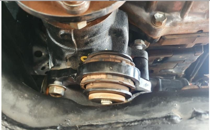
9. Assemble the new left and right cradle arms as shown. Use a hammer to knock the poly bushes into the front of the new left side cradle, and the front and rear of the new right side cradle. Put a small amount of grease and knock the sleeves into the poly bushes ensuring the poly bushes are held against something to prevent them unseating from the arms. You can also do this in a vice
