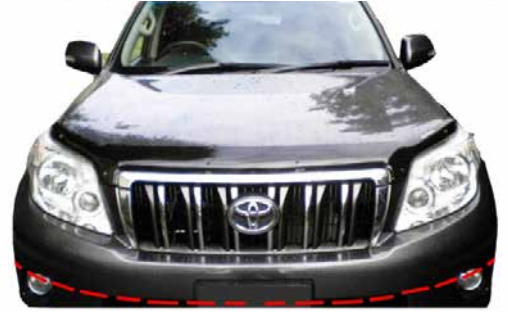
Mark from bottom edge of template across to top of grill section on bumper to cut
