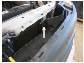
8. Reach in behind the grill and unclip the lower tabs and remove the grill.
