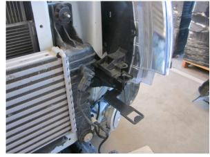
18. Install the LH and RH triangular bracket supports first on the outside of each chassis rails as per page 3 diagram. Insert the captive nut (item 3) through the front of the chassis and insert nuts and washers. The LH bracket can also be bolt at the back.
