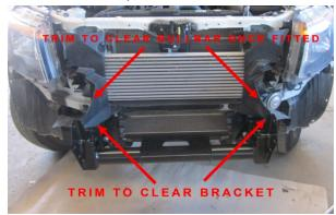
22. Reinstall the grill. The tabs on the grill go down from the top into the newly fitted brackets.
