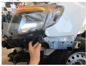
17. Install the New grill support brackets (item 16) onto the spare bolt hole on the inside near the bottom of the headlight, using the 2 x black dome head bolts supplied.
