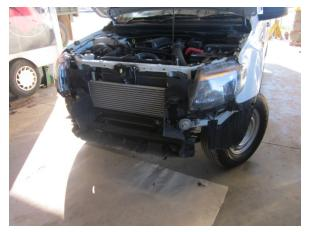
12. Remove the plastic front panel and remove the steel bumper bar re-enforcement. Do not discard these bolts they are used to attach the bullbar bracket.
