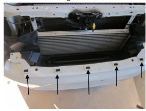
9. Remove all wheel arch liner bolts attaching the wheel arch liner to the bumper, also remove the upper bumper bolt.
