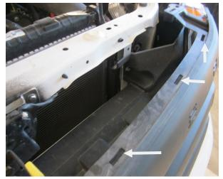
5. Remove the clip and bolt on each side of the grill holding the lower section of the grill and plastic shrouds.
