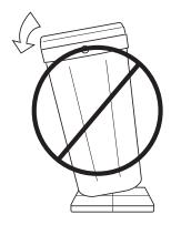
Do not tip the barrel to get the water out. This can stress the base and cause leaking.
