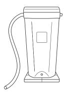
To prevent the barrel from tipping over Make sure your block base is wider than the bottom of the rain barrel.
