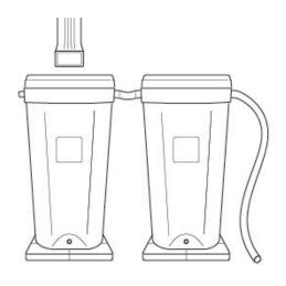
**Daisy chaining multiple rain barrels:** Link two or more barrels so the over flow will drain into the additional barrel(s).
