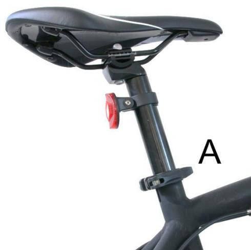
The saddle can be tilted and also adjusted in the longitudinal direction for best fit. This may be adjusted by loosening the hex screw located under the saddle. Adjust to the desired position then tighten.
