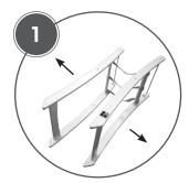
1a. Seperate the two leg panels as shown.
