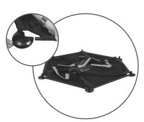
**NOTE:** The 2 x Lower Joints (with Pop-Pin holes) MUST be used at opposite corners.
