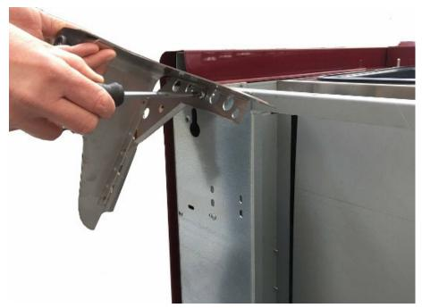
9. Attach the feet using a phillips head screwdriver to fasten the screws and washers included with the range. 10. Set the range upright. NOTE: The range can now be set on its feet directly on the floor. If the range needs to be moved further, be sure not to drag it.
