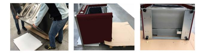
8. Tilt the range and set it down so its back is on the floor NOTE: In this step, no part of the range should touch the floor directly and must be buffered by padding. This is to prevent damage to both the range and the floor.
