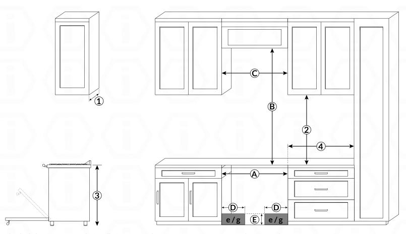
The shaded area represents the installation area for the connections
