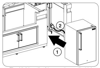
Fig. 14-4 Install refrigerator (as applicable)
