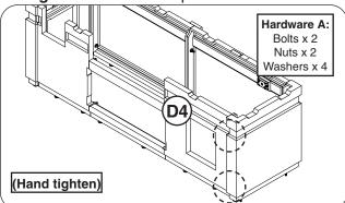
Fig. 10-4 Assemble front wall (right piece)
