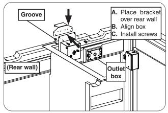
Fig. 14-2 Install power supply box
