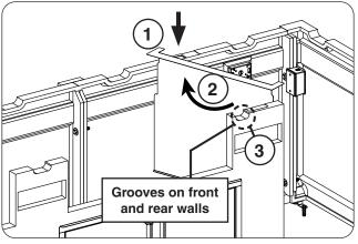
Fig. 14-1 Place heat shield (as applicable)
