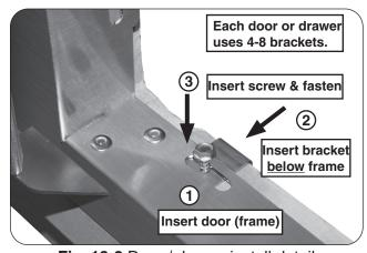
Fig. 13-2 Door / drawer install detail
