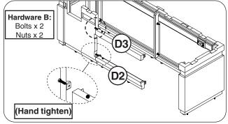
Fig. 10-3 Assemble top and bottom beams
