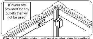
Fig. 9-4 Right side wall and outlet box installed
