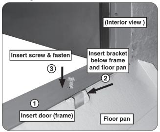
Fig. 13-3 Door / floor pan install detail
