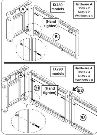
Fig. 9-2 Assemble left side and rear wall
