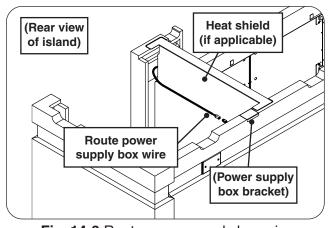
Fig. 14-3 Route power supply box wire
