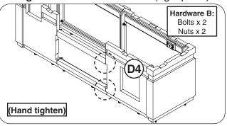
Fig. 10-5 Assemble top and bottom beams
