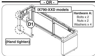
Fig. 10-2 Assemble front wall (left piece)
