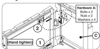
Fig. 9-3 Assemble right side wall and outlet box
