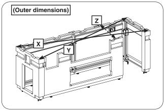
Fig. 11-2 Square unit (then tighten all bolts)
