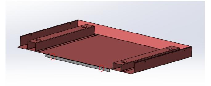
4. Install the frame with brackets to the cabinetry. Use the 4 holes (circled below in RED) to mount to the front of the cabinetry.
