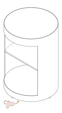
The Arteflame draws in air through the bottom of the base so make sure you have a 3/8" to 1/2" air gap under the base.
