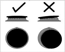
3. Place the grates on the rangetop. For maximum stability, these grates should only be used in their proper position. Because of the varied burner sizes, the side grates cannot be exchanged nor can any of the grates be rotated front to back.
