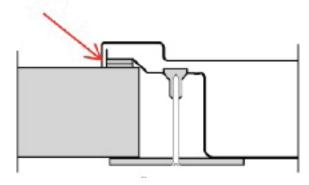
Reinsert the cooktop into the countertop opening. Lift the entire cooktop to make adjustments. Attach the brackets to the bottom of the unit. Insert the clamping screws into the brackets. Use a screw-driver to tighten the clamping screws against the underside of the countertop. Refer to the illustration below. Do not overtighten screws.
