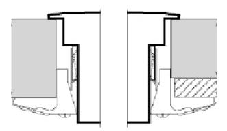
IMPORTANT NOTE: Do not seal the cooktop to the countertop. It must be removed if service is necessary. GAS PRESSURE REGULATOR Install the gas pressure regulator with the arrow on the regulator pointing up toward the unit and in a position where you can reach the access cap.
