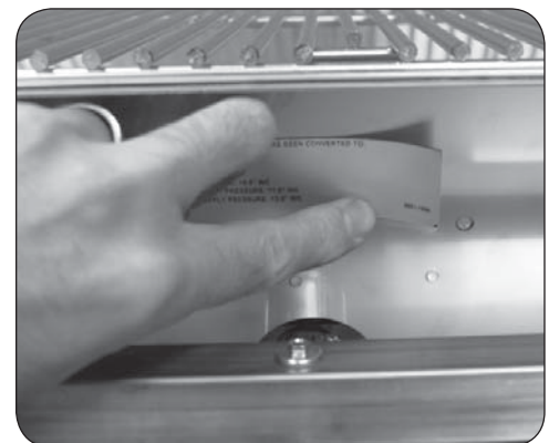
Fig. 4-3 Apply the conversion label
