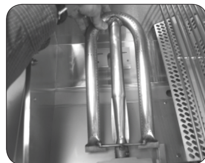
Fig. 1-2 Remove the burner
