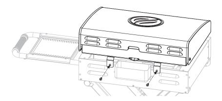
STEP 13 Use two (2) M6x16 screws (found within the hood handle) to install the hood handle and two (2) handle grommets to the hood.
