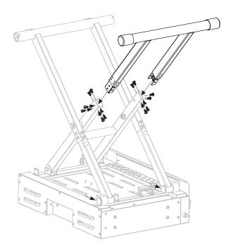
**STEP 05** Use four (4) M6x28 bolts, two (2) M6x45 bolts, and six (6) M6 nuts to install the two (2) anti-tippers onto the wheeled leg assembly crossbar.
