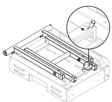
**STEP 03** Raise the legs. Use twelve (12) M6x12 bolts to install the upper legs onto the wheeled leg assembly.
