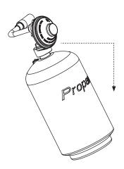
If the liquid level of the propane is above the regulator, the regulator will frost.
