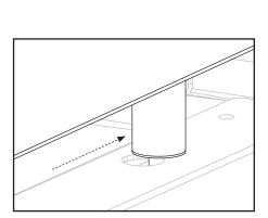
Ensure that all four pins are seated in the holes, then push the griddle top forward to lock the griddle in place.
