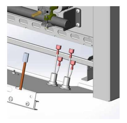
5. Before removing the main burner orifices, take a visual note as to how far the orifice is installed onto the valve body. The orifices are removed with a 1/2" deep socket wrench. Use even pressure to break loose the old orifice and remove from the valve.
