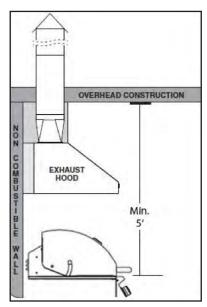
**Combustible Overhead Construction:** Exhaust hood required.
