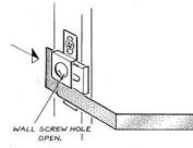
Once the picture is locked on the wall, you can only remove it with the *Release Tool*.
