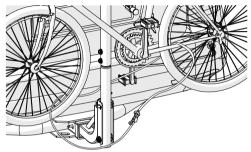
To help deter theft, thread securing cable around frame of rack and through spokes of front wheel, then above and through frame and spokes of rear wheel. Align grommet end with locking pin as shown. Apply lock.
