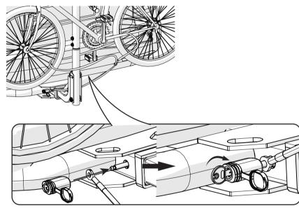
**Step 8:** Take out safety pin from the base of the rack and tilt it for rear access.
