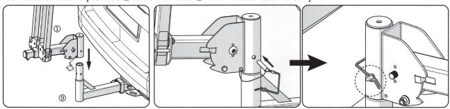
STEP 3: Secure the rotatable post tube ① with the locking knob.
