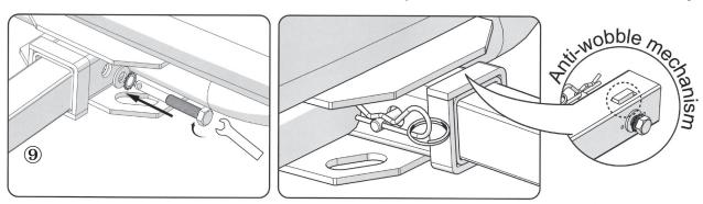
Use wrench to tighten the safety bolt. Anti-wobble mechanism is functioning when the safety bolt is tightened.
