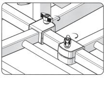
Install wheel holder stop screws & internal toothed lock washers with Phillips screwdriver.
